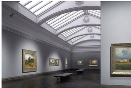
Ideal for museums with a high level of daylight: Eclipse InTrack spotlights in tunable white: their light colour can be infinitely adjusted – via DALI or wireless, via Casambi Bluetooth or Zigbee 3.0.
